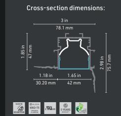
The 8540 Pro profile is designed to disappear into the structure, merging the light source with the surface and house our Luxline serie of 120V LED engine tape. Its 90° edge on one side makes it ideal for contour lighting application. Its refined look harmonizes perfectly with any project.
